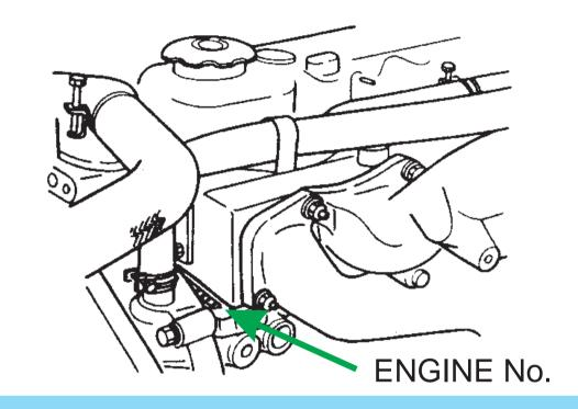
DIESEL ENGINE No. STAMPED ON THE FRONT PART OF THE CYLINDER BODY
